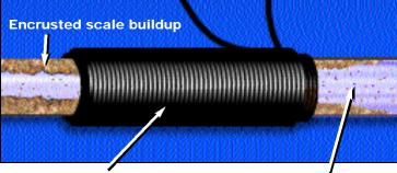
Signal Coil producing magnetic field inside the pipe. The resulting induced, oscillating electric field provides the necessary molecular agitation for scale and bio-film prevention and removal
