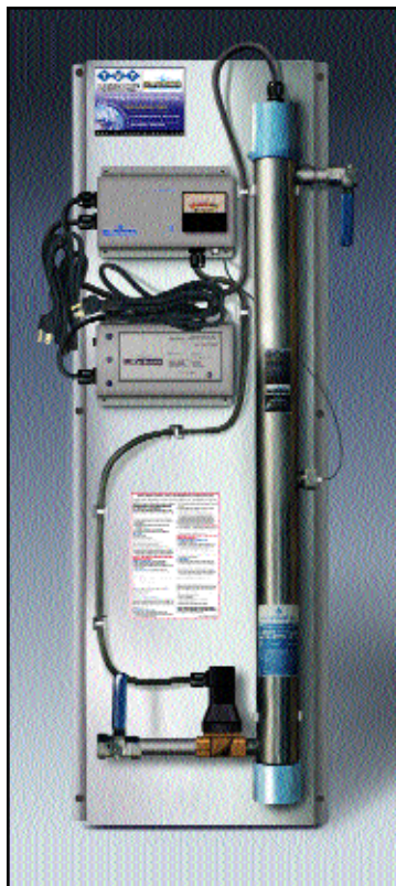
TWT-UVC-1500 (15 GPM) Ultraviolet Disinfection/Purification System Mounted on St/St frame with Manual Shut-Off Valves, Alarm, UV Monitor and Automatic Solenoid Valve Size: 20"W X 55"H 10"D Available 120V/60 Hz or 230V/50 Hz
