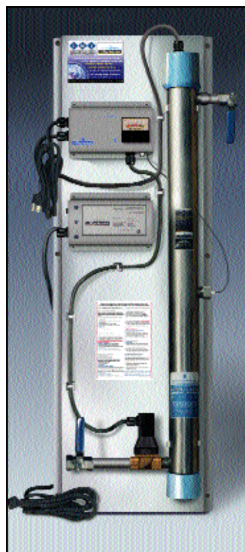
TWT-UVC-3000 (30 GPM) Ultraviolet Disinfection/Purification System Mounted on St/St frame with Manual Shut-Off Valves, Alarm, UV Monitor and Automatic Solenoid Valve Size: 20"W X 55"H 10"D Available 120V/60 Hz or 230V/50 Hz
