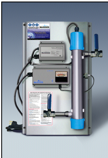
TWT-UVC-250 (4 GPM) Ultraviolet Disinfection/Purification System Mounted on St/St frame with Manual Shut-Off Valves, Alarm and UV Monitor Size: 18"W X 26"H 6"D Available 120V/60 Hz or 230V/50 Hz
