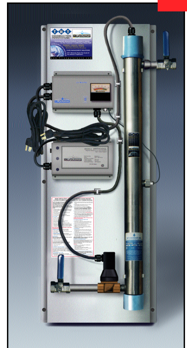
TWT-UVC-1200 (12 GPM) Ultraviolet Disinfection/Purification System Mounted on St/St frame with Manual Shut-Off Valves, Alarm, UV Monitor and Automatic Solenoid Valve Size: 20"W X 44"H 10"D Available 120V/60 Hz or 230V/50 Hz
