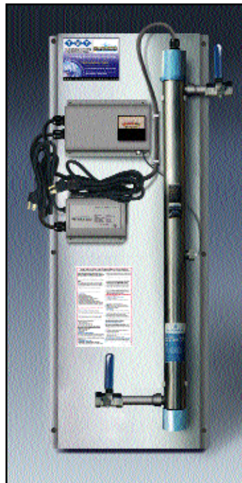
TWT-UVC-700 (8 GPM) Ultraviolet Disinfection/Purification System Mounted on St/St frame with Manual Shut-Off Valves, Alarm and UV Monitor Size: 20"W X 20"H 44"D Available 120V/60 Hz or 230V/50 Hz
