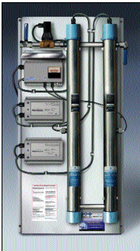
TWT-UVC-6000 (100GPM) Ultraviolet Disinfection/Purification System Mounted on St/St frame with Manual Shut-Off Valves, Alarm, UV Monitor and Automatic Solenoid Valve Size: 25"W X 55"H 10"D Available 120V/60 Hz or 230V/50 Hz
