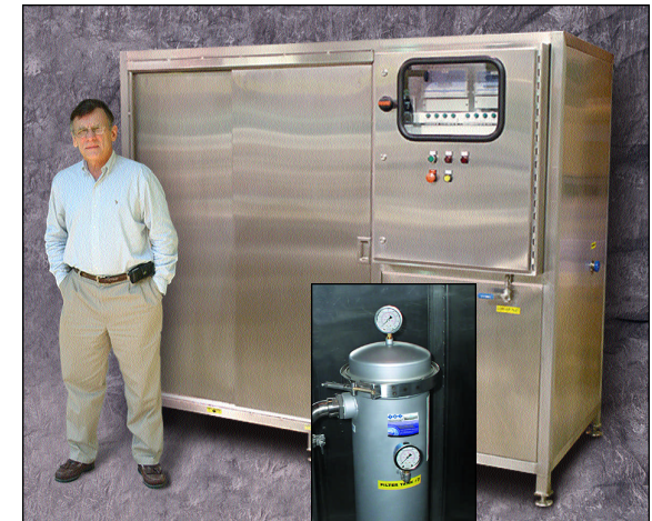
Triple Quattrra 100 UV system configured to provide more exposure to the UV light, ensuring a higher kill rate of the bacteria.
