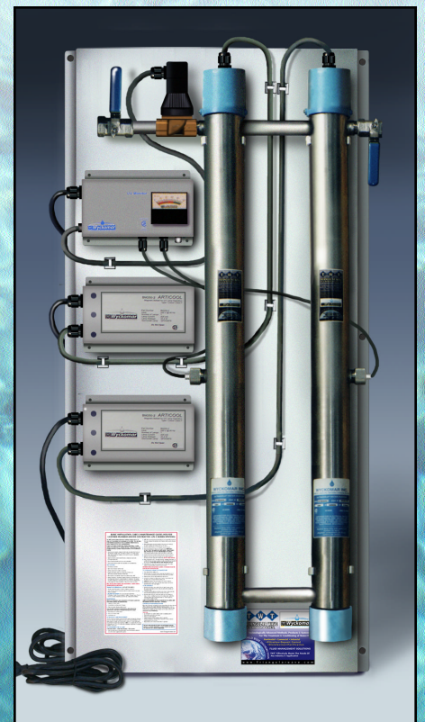
TWT-UVC-5000 (50 GPM) Ultraviolet Disinfection/Purification System Mounted on St/St frame with Manual Shut-Off Valves, Alarm, UV Monitor and Automatic Solenoid Valve Size: 55"W X 25"H 10"D Available 120V/60 Hz or 230V/50 Hz
