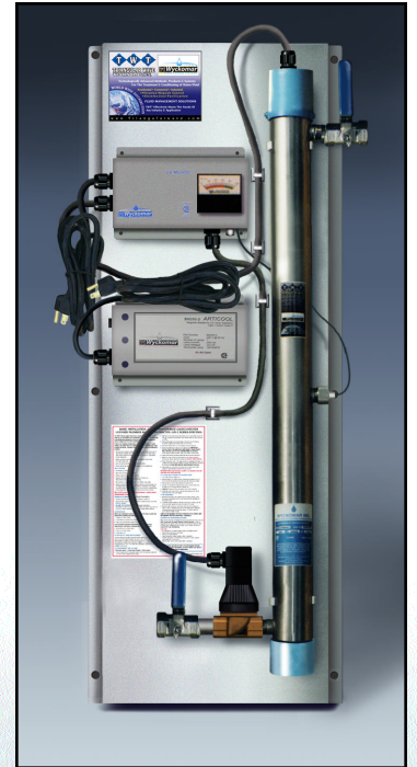
TWT-UVC-1200 (12 GPM) Ultraviolet Disinfection/Purification System Mounted on St/St frame with Manual Shut-Off Valves, Alarm, UV Monitor and Automatic Solenoid Valve Size: 44"W X 20"H 10"D Available 120V/60 Hz or 230V/50 Hz
