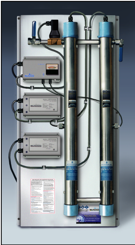
TWT-UVC-6000 (100GPM) Ultraviolet Disinfection/Purification System Mounted on St/St frame with Manual Shut-Off Valves, Alarm, UV Monitor and Automatic Solenoid Valve Size:55"W X 25"H 10"D Available 120V/60 Hz or 230V/50 Hz
