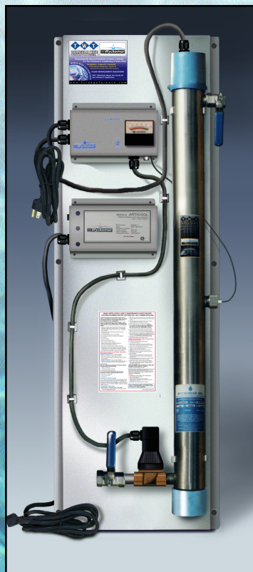
TWT-UVC-3000 (30 GPM) Ultraviolet Disinfection/Purification System Mounted on St/St frame with Manual Shut-Off Valves, Alarm, UV Monitor and Automatic Solenoid Valve Size: 55"W X 20"H 10"D Available 120V/60 Hz or 230V/50 Hz
