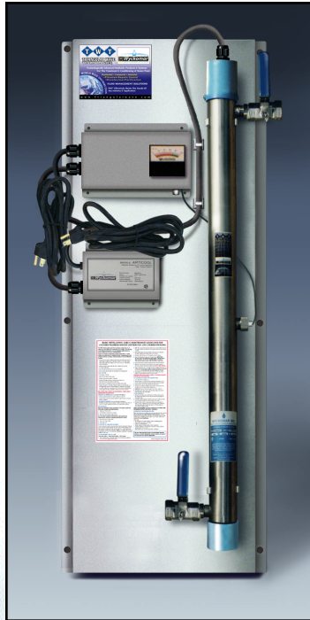
TWT-UVC-700 (8 GPM) Ultraviolet Disinfection/Purification System Mounted on St/St frame with Manual Shut-Off Valves, Alarm and UV Monitor Size: 44"W X 20"H 10"D Available 120V/60 Hz or 230V/50 Hz
