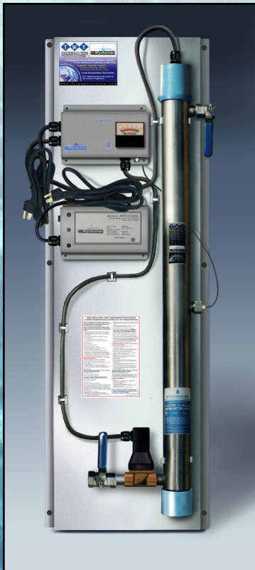
TWT-UVC-1500 (15 GPM) Ultraviolet Disinfection/Purification System Mounted on St/St frame with Manual Shut-Off Valves, Alarm, UV Monitor and Automatic Solenoid Valve Size: 55"W X 20"H 10"D Available 120V/60 Hz or 230V/50 Hz
