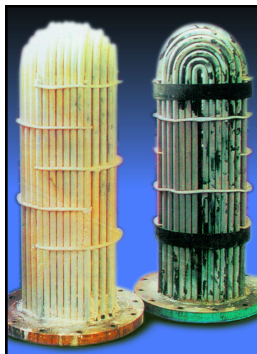
Encrusted Heat Exchangers
