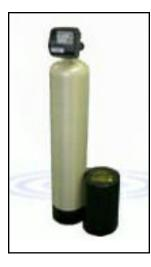
TWT-RE-30 Maximum Iron Removal Capacity: 30 p.p.m. Flow rate: 30 Liters per minute Maximum Iron Removal Capacity: 30 p.p.m. Filter Medium: Fine birm Plumbing: 1" and 1" N.P.T. In-Out Back-wash Connection: 3/4" N.P.T. Size: 52" high X 12" diameter Weight: 80 lbs.
