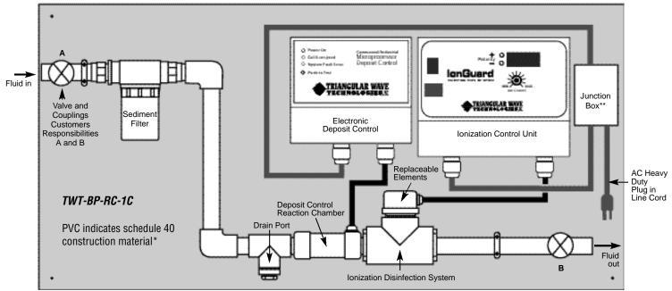
Schematic rendering of TWT Bypass Treatment System
