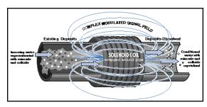
Signal coil producing magnetic field inside the pipe. The resulting induced, oscillating electric field provides the necessary molecular agitation for scale and biofilm prevention and removal.
