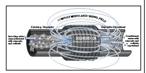
Signal coil producing magnetic field inside the pipe. The resulting induced, oscillating electric field provides the necessary molecular agitation for scale and biofilm prevention and removal.
